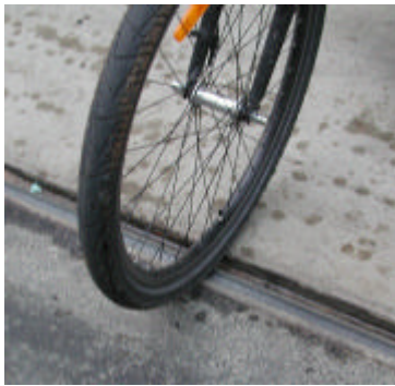
The best angle to cross tram tracks is at right angles - as shown
